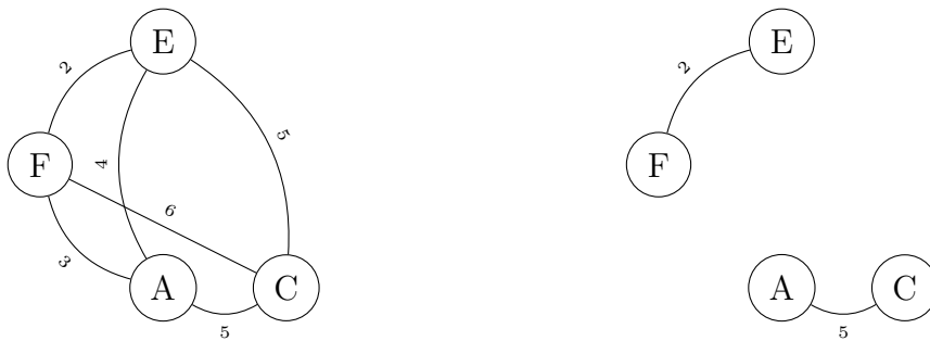
Figure 11: Finding minimum perfect matching M^* of subgraph O .
