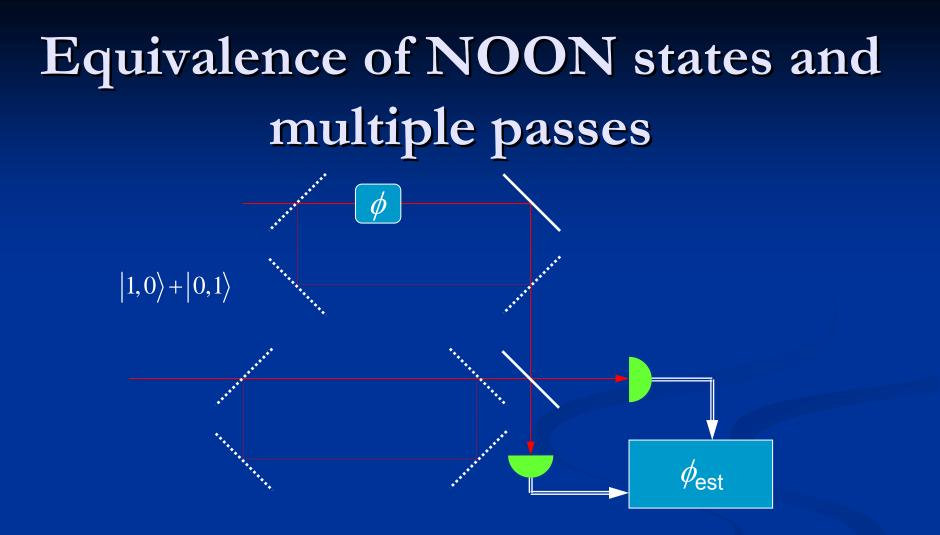
Electro-optic switches pass single photon through phase shift at times  $t_1 - \Delta t, t_2 - \Delta t, \dots t_N - \Delta t.$
